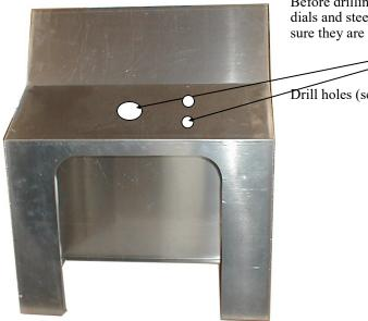
Before drilling holes to mount dials and steering system make sure they are properly laid out.
